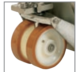
Wheels with rubber-sealed bearings.
