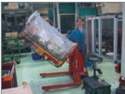
The straddle model makes it possible to handle closed pallets. The Logitilt being used in the component industry.
